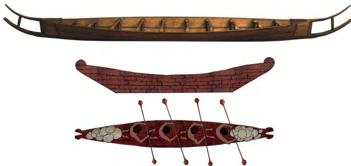
Figure 4.2. Comparison of sewn-plank boats in Scandinavia and California. The model of Hjortspring boat is above, while a drawing of a Chumash plank canoe is depicted below. Both ships are shown scaled to size, with Hjortspring having an interior length of 13.6 m while large Californian canoes were up to 9 m in length. (Hjortspring boat model credited to Richard Potter; used with permission; California canoe drawing by Mikael Fauvelle and Jaymee Ngermwichit).
